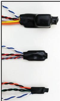
DESI-R: A single form-C relay output for controlling electromechanical device controller
